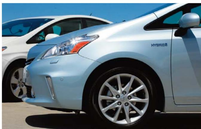
This hybrid has both a petrol and an electric motor
